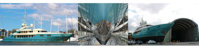
The 47 metre ISA built motor yacht was constructed in Italy in 2006 in steel and aluminium to Lloyds International Class Rules. The yacht is MCA and RINA compliant.
